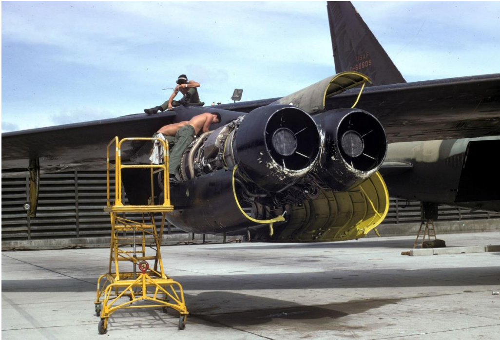
Figure 19. Maintainers work the outboard engines of a B-52D at Guam during LINEBACKER II. Image Source: United States Air Force.
