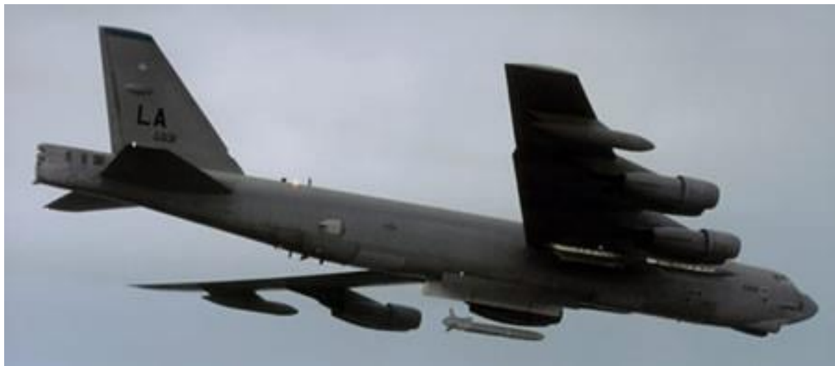
Figure 2. Second Bomb Wing B-52 H from Barksdale AIR FORCE BASE launching a AGM-86C CALCM. Source: Federation of American Scientists file photo.
